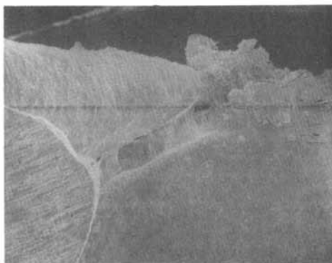
Figure 1. SEM photomicrographs of the filler metal and grinding swarf on a Vehicle Information Number (VIN) Tab (275 \times )
