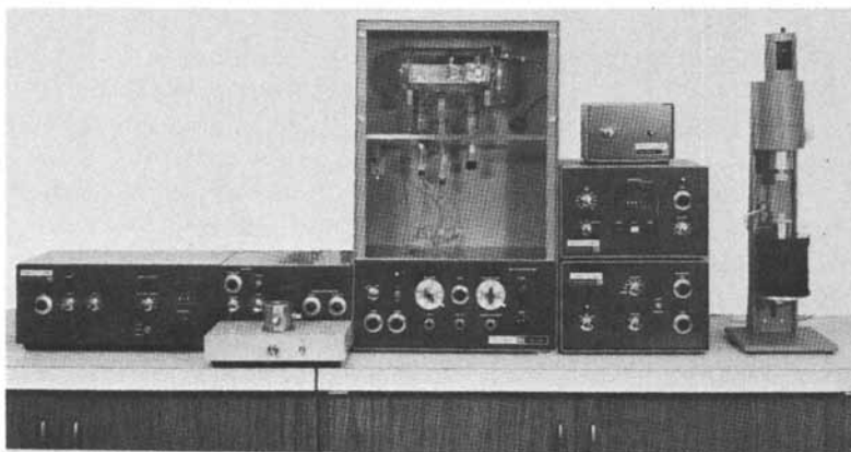
Figure 1. The Perkin-Elmer laboratory for thermal analysis. From left to right: the DSC-1B differential scanning calorimeter with evolved gas analyzer, the TGS-1 thermobalance (top to bottom), the recorder chart control, model UU-1 temperature programmer control, and model TMS-1 control unit. At right is the model TMS-1 thermomechanical analyzer.
