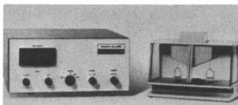
Figure 3. Model AD-2 precision electronic microbalance (capacity 5g; sensitivity 0.1 \mu g)
